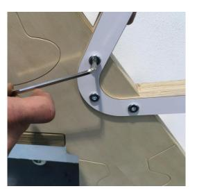
**1.3** Now tighten the screw on both sides using a 5 mm allen key. Repeat the insertion of the screw, the fastening of the the screw heads and the even tightening for all drillings of the module.
