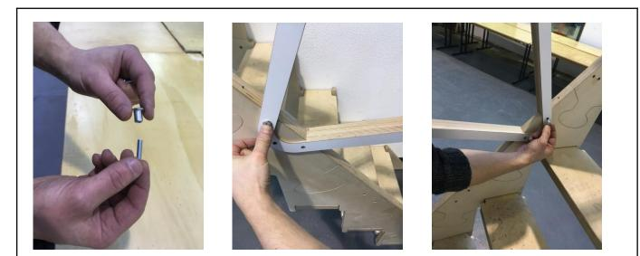
**1.2** Assemble a screw head with a grub screw. These can now be pressed through the holes. On the opposite side, the module should now be secured by another screw head.
