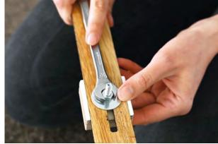
② Then tighten the screw until the multiplex block can no longer be shifted during the assembly of the staircase.
